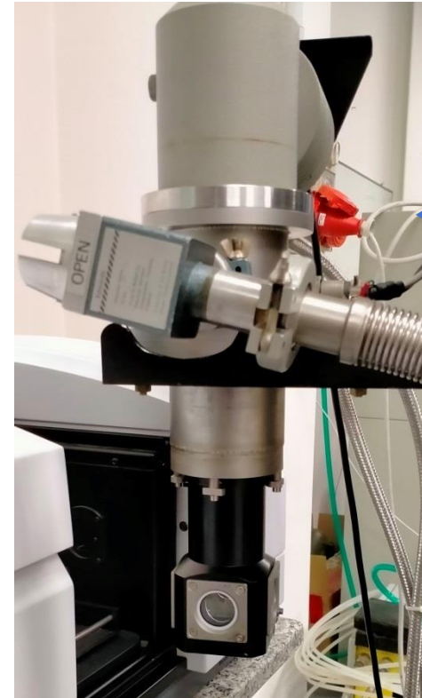
Left: Low-temperature absorption setup. On the background, there is the Cary 5000 spectrometer, into which we inserted cryostat connected to a vacuum pump, and a temperature controller; Top: Detail of the cryostat itself.
