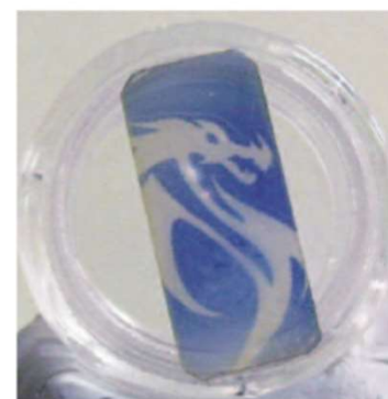
▲ Dragon's picture recorded on porous glass loaded with Rb. The sample region exposed to light becomes blue due to the increase of the number of Rb nano-particles with respect to the equilibrium condition in the dark.
