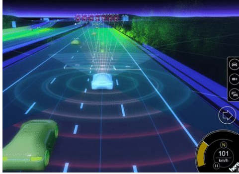
Figure 7: Example of how a LIDAR gathers information in an autonomous vehicle Credit: Jonathan Hui
