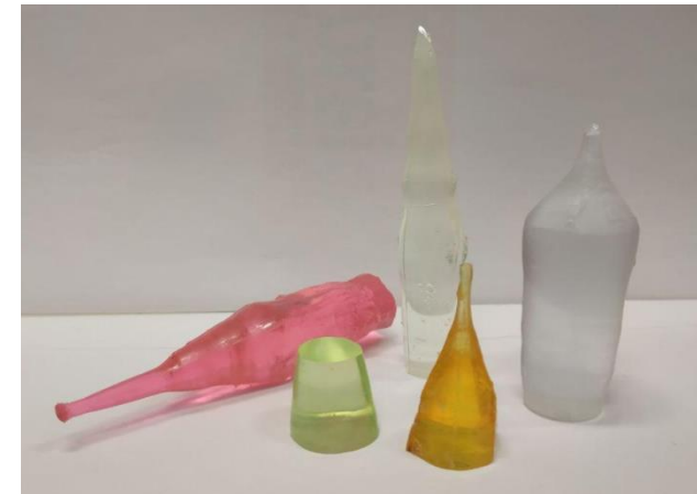
Left: boules of fluoride monocrystals doped with rare earth elements (from www.megamaterials.it )
